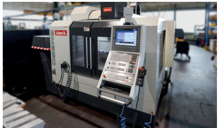
AWEA BM 850 X: 850 mm, Y: 600 mm, Z: 600 mm Heidenhain TNC 530
