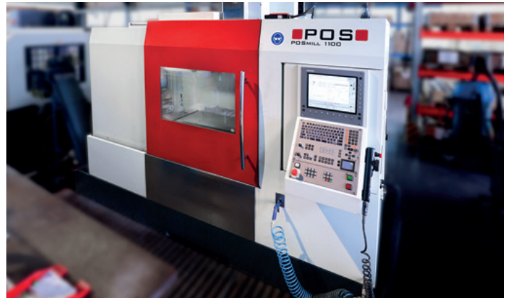
POS 1100E X: 1.100 mm, Y: 550 mm, Z: 520 mm Heidenhain TNC 530
