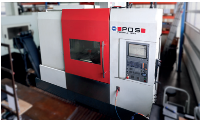
POS 1100E X: 1.100 mm, Y: 600 mm, Z: 520 mm Heidenhain TNC 530
